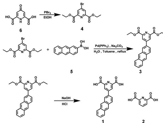
Scheme 1 Synthetic scheme of **1** and the structure of **2**.
