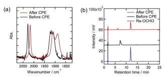
Fig. 11 (a) FT-IR spectra and (b) UHPLCs of the Re(i) complexes before and after electrolysis at -1.82 V with the existence of TPAHBF4 (25 mM) under a 100% CO<sub>2</sub> atmosphere in DMF-TEOA containing Et<sub>4</sub>NBF<sub>4</sub> (0.1 M) as the supporting electrolyte (black lines: before electrolysis, red lines: after electrolysis). Measurement conditions were the same as those in Fig. 9.
