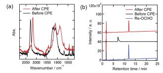
Fig. 12 (a) FT-IR spectra and (b) UHPLCs of the Re(i) complexes before and after electrolysis at -1.82 V with the existence of TPAHBF<sub>4</sub> (25 mM) under a 1% CO<sub>2</sub> atmosphere in DMF-TEOA containing Et<sub>4</sub>NBF<sub>4</sub> (0.1 M) as the supporting electrolyte (black lines: before electrolysis, red lines: after electrolysis). Measurement conditions were the same as those in Fig. 9.
