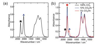
Fig. 1 FT-IR spectra of the Re(i) complexes (5.0 mM) in a DMF-TEOA (5 : 1 v/v) solution containing 0.1 M  $\rm Et_4NBF_4$  after purging with Ar (a), and Ar containing various concentrations of  $\rm CO_2$  (b). Black asterisk (\*), blue triangle ( $\blacktriangle$ ) and red circle ( $\bullet$ ) display the peaks which correspond to Re-DMF<sup>+</sup>, Re-TEOA, and Re-CO<sub>2</sub>TEOA, respectively.
