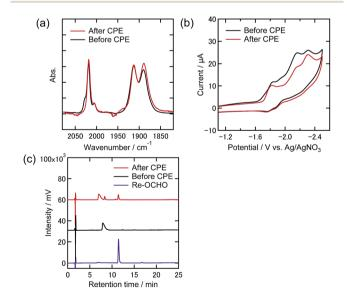
Fig. 10 (a) FT-IR spectra, (b) CVs, and (c) UHPLCs of the Re(I) complexes before and after electrolysis at -1.82 V under a 1% CO<sub>2</sub> atmosphere in DMF-TEOA containing  $Et_4NBF_4$  (0.1 M) as the supporting electrolyte (black lines: before electrolysis, red lines: after electrolysis). Measurement conditions were the same as those in Fig. 9.
