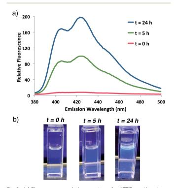
Fig. 2 (a) Fluorescence emission spectrum for ATRP reaction shown in Scheme 1 at indicated times following 337 nm excitation. (b) Photographs of the reaction at indicated times illuminated by a handheld UV light (365 nm).
