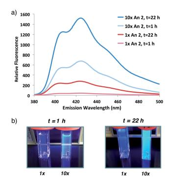
Fig. 3 (a) Fluorescence emission spectrum of initial anthracene: PEG 2:5 molar ratio  $(1\times,1:9300)$  or 10-fold increase in An  $2(10\times,1:930)$  co-polymerization at indicated times following 337 nm excitation. (b) Photographs of sample illuminated by hand-held UV light (365 nm).
