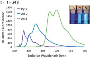
Fig. 4 Emission spectra and photographs of pyrene, anthracene and acridine co-polymerization reactions following excitation at 337, 371 or 431 nm, respectively, at 1 h (a) or 24 h (b).
