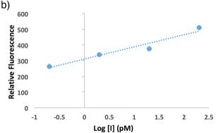
Fig. 6 (a) Emission spectra and photograph of anthracene ATRP copolymerization at 60  $^{\circ}$ C with indicated concentrations of initiator 4 at 1 h of reaction time following excitation at 371 nm. (b) Plot of relative fluorescence intensity at 426 nm *versus* of initiator concentration from the reaction in (a).
