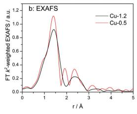
Fig. 5 Vtc-XES (a) and FT  $k^2$ -weighted EXAFS (b) spectra of Cu-0.5 and Cu-1.2 catalysts measured under dry air at 350 °C.
