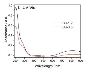
Fig. 3 Ex situ FT  $k^2$ -weighted EXAFS spectra (a, uncorrected for the phase shift) and DR UV-vis (b) spectra of Cu-0.5 and Cu-1.2 catalysts.
