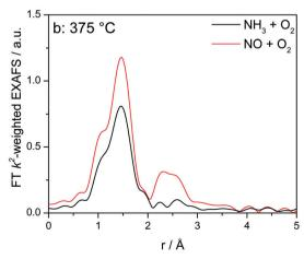
Fig. 9 Operando FT  $k^2$ -weighted EXAFS measured on Cu-0.5 in the temperature regions with (a) low NO $_x$  conversion (200 °C) and (b) NO $_x$  conversion onset (375 °C). Conditions: 1000 ppm NO or 1000 ppm NH $_3$ , 10% O $_2$ , 1.5% H $_2$ O/He, GHSV 200 000 h $^{-1}$ .
