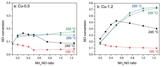
Fig. 2 Conversion of NO during NH<sub>3</sub>-SCR of NO<sub>x</sub> at different NH<sub>3</sub>: NO ratios over (a) Cu-0.5 and (b) Cu-1.2 catalysts. Conditions: 1000 ppm NO, 100-1250 ppm NH<sub>3</sub>, 10% O<sub>2</sub>, 2% H<sub>2</sub>O, balance N<sub>2</sub>, GHSV 200 000 h<sup>-1</sup>.
