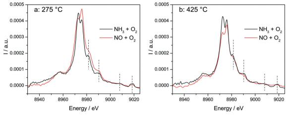
Fig. 10 In situ vtc-XES measured on Cu-1.2 at (a) 275 °C and (b) 425 °C. Conditions: 1000 ppm NO or 1000 ppm NH<sub>3</sub>, 10% O<sub>2</sub>, 1.5% H<sub>2</sub>O, balance He, GHSV 200 000 h<sup>-1</sup>.
