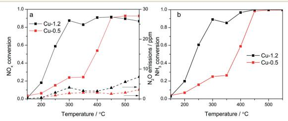
Fig. 1 Conversion of  $NO_x$  and production of  $N_2O$  (a), and conversion of  $NH_3$  (b) measured during  $NH_3$ -SCR over the tested Cu-zeolites measured in the laboratory plug-flow reactor. Conditions: 1000 ppm NO, 1000 ppm  $NH_3$ , 10%  $O_2$ , 5%  $H_2O$ , balance  $N_2$ , GHSV 200 000  $h^{-1}$ .
