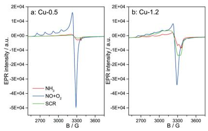
Fig. 12 In situ EPR spectra of (a) Cu-0.5 and (b) Cu-1.2 samples measured at 250 °C in: 2000 ppm NH $_3$ /Ar (red line); 2000 ppm NO, 10% O $_2$ /Ar (blue line) and 2000 ppm NH $_3$ , 2000 ppm NO, 10% O $_2$ /Ar (green line).
