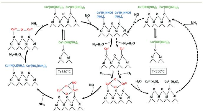
Scheme 2 Involved species and mechanistic aspects of  $NH_3$ -SCR over low and highly loaded Cu-SSZ-13 samples at temperatures below (right side) and above (left side) the seagull profile minimum (unbalanced reactions for better overview on evolved species). An approximate number of adsorbed  $NH_3$  or  $H_2O$  molecules at low and high temperature is suggested based on the calculated coordination numbers in Table 2 and on previously published results.<sup>76</sup>
