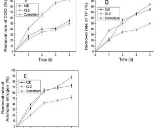
Fig. 5 The pollutant removal performances of single Chlorella sorokiniana XJK, single Aspergillus sp. XJ-2 and the consortium. (a) Removal of COD; (b) removal of TP; (c) removal of ammonia nitrogen.
