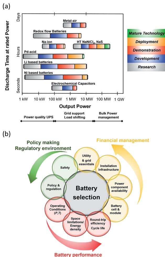
Fig. 2 (a) Current status of Battery Energy Storage Technologies (BESS). Data taken from ref. 17 and 18. Metal air batteries: Zn-air and Li-air; RFB: Zn-Ir, Zn-Br<sub>2</sub>, Zn-NiO, Ir-Cr, VRFB. Pb-acid batteries: advanced and valve-regulated. Li based batteries: LTO, LCO, LFP, NMC, NCA and Li-polymer. Ni based batteries: Ni-Cd, Ni-Fe. (b) Criteria for BESS selection.
