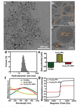
Fig. 1 (a) TEM image, (b) enlarged TEM image and (c) HRTEM image of Fe<sub>3</sub>O<sub>4</sub>-Pd JNPs. (d) Hydrodynamic size of Fe<sub>3</sub>O<sub>4</sub>-Pd JNPs. (e) Zeta potential of Pd NSs,  $Fe_3O_4$  NPs and  $Fe_3O_4$ -Pd JNPs. (f) UV-vis-NIR absorption spectra of Pd NSs, Fe<sub>3</sub>O<sub>4</sub> NPs and Fe<sub>3</sub>O<sub>4</sub>-Pd JNPs. (g) Magnetization hysteresis loops of Fe<sub>3</sub>O<sub>4</sub>-Pd JNPs.
