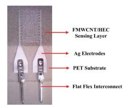
Fig. 5 Photograph of the printed sensor.
