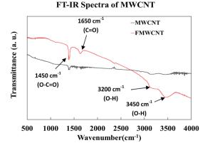
Fig. 11 FT-IR spectra of the MWCNTs and FMWCNTs.
