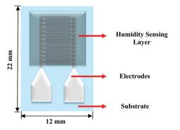
Fig. 3 Schematic of the humidity sensor (not to scale).
