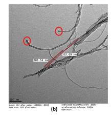
Fig. 9 TEM micrographs of FMWCNTs showing (a) a diameter of 10-20 nm (marked in red circles) and (b) a length of 0.1-1 µm.
