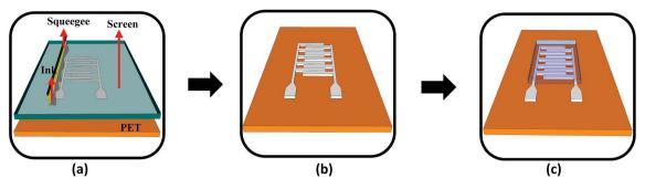
Fig. 4 (a) Screen printing of Ag ink on the PET substrate, (b) screen printed IDTs and (c) gravure printing of the MWCNT/HEC ink on the electrodes (not to scale).
