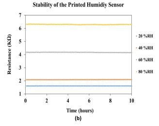
Fig. 16 (a) Transient response of the printed humidity sensor and (b) stability of the printed humidity sensor.
