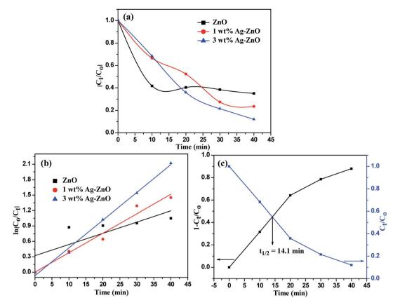
Fig. 7 (a) Comparative photocatalytic degradation of chlorpyrifos pesticide using bare ZnO NPs and 1 and 3 wt% Aq-ZnO, (b)  $\ln(C_0/C_t)$  vs. time (min) curve for photodegradation of chlorpyrifos, and (c) half-life estimation for degradation of pesticide using 3 wt% Ag-ZnO
