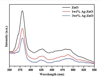
Fig. 8 PL spectra of bare ZnO NPs and 1 and 3 wt% Aq-ZnO nanocomposites.
