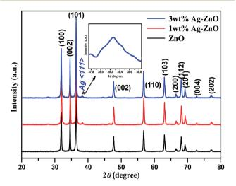
Fig. 2 XRD patterns of bare ZnO NPs and 1 and 3 wt% Aq-ZnO hybrid composites
