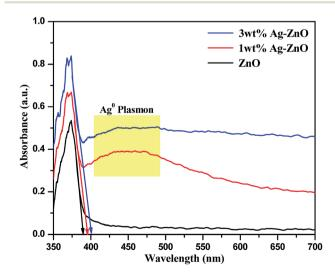
Fig. 1 DRS of bare ZnO NPs and 1 and 3 wt% Aq-ZnO hybrid composites
