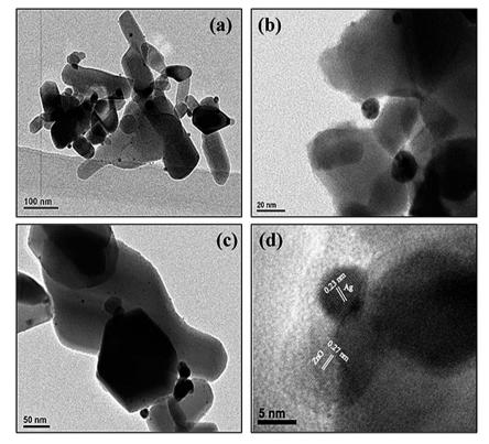
Fig. 3 TEM images (a and b) for 1 wt% Aq-ZnO and (c and d) 3 wt% Aq-ZnO.
