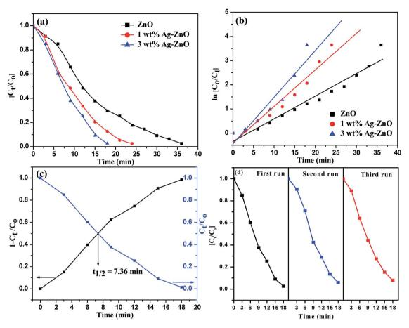
Fig. 6 (a) Comparative photocatalytic degradation of Rh-B dye using bare ZnO NPs and 1 and 3 wt% Ag-ZnO, (b)  $\ln(C_{\rm o}/C_{\rm t})$  vs. time (min) curve for photodegradation of Rh-B, (c) half-life estimation curve for degradation of Rh-B dye using 3 wt% Ag-ZnO, and (d) reusability of 3 wt% Ag-ZnO photocatalyst for decomposition of Rh-B dye for three consecutive cycles.
