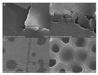
Fig. 4 AAO substrates in SEM micrographs. (A and B) CSVD process has prioritized pores, cracks, and even concave surfaces over flat and open planes. (C) Heterogenous CSVD process where feature filling and subsequent planarization proceeded further along cracks than over the surface. (D) Locally successful pore filling.
