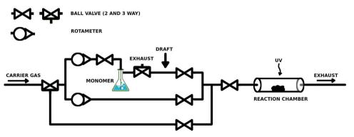
Fig. 1 The experimental reactor line setup.
