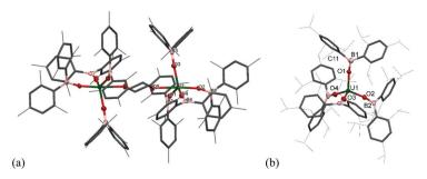
Fig. 2 Displacement ellipsoid drawing of the molecular structure of (a) 2<sup>m</sup>·diox and (b) 2<sup>t</sup>·C<sub>7</sub>H<sub>8</sub>. Thermal ellipsoids are displayed at 50% probability. Lattice solvent and hydrogen atoms omitted, and aryl substituents are depicted as wireframe and capped sticks for clarity.
