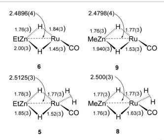
Scheme 3 Summary of key distances in  $[Ru(IPr)_2(CO)(H)_2ZnR][BAr^F_4]$  and  $[Ru(IPr)_2(CO)(\eta^2-H_2)(H)_2ZnR][BAr^F_4]$  (R = Et, Me).
