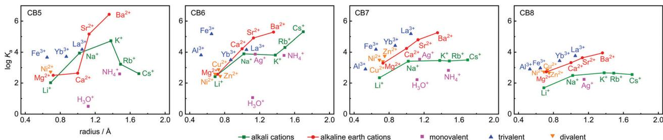
**Fig. 2** Plots of  $\log K_a$  vs. cation radius for different CBn.
