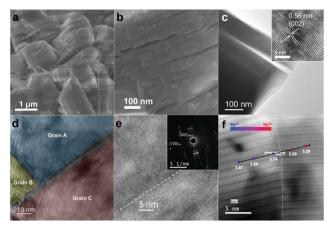
Fig. 3 (a) and (b) SEM images and (c) TEM image of the nanostructured P2-Na $_{2/3}$ MnO $_2$  (Inset: Magnified HRTEM image). HRTEM images of (d) three neighboring grains: A, B, and C (e) the interface region with a SAED pattern (inset) indicating the different orientations. (f) High-angle annular dark-field STEM image of the interface region with an EELS line scan.
