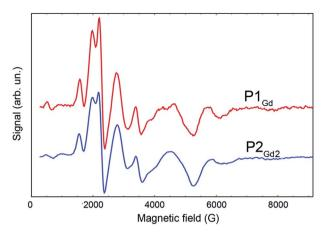
Fig. 6 EPR spectra comparing the derivative of the free-induction-decay-detected absorption of  $P1_{Gd}$  (red line) and  $P2_{Gd2}$  (blue line). The spectra were acquired at X-band frequency (9.4 GHz) at 3 K in a 1 : 1 mixture of dichloromethane and toluene.
