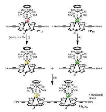
Fig. 1 General structure of  $P1_{Ln}$  and the synthetic route of the heterometallated dimer  $P2_{Dy-Tb}$  (Ln = Tb). Reaction conditions: (i) TBAF, CHCl<sub>3</sub>/CH<sub>2</sub>Cl<sub>2</sub>, 50%; (ii) TBAF, CHCl<sub>3</sub>/CH<sub>2</sub>Cl<sub>2</sub>, 44%; (iii) Pd(PPh<sub>3</sub>)<sub>2</sub>Cl<sub>2</sub>, Cul, 1,4-benzoquinone, toluene $^{j}$ Pr<sub>2</sub>NH, 48%. Ln = Y, Gd, Tb, Dy; TIPS = triisopropylsilane; CPDIPS = cyanopropyldiisopropylsilane; Ar = 3,5-bis(tert-butyl)phenyl.
