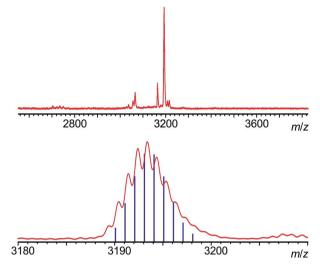
Fig. 2 MALDI-TOF mass spectrum of  $P2_{Dy-Tb}$ , acquired with a dithranol matrix. The absence of homodinuclear species (which would fall at 3188 and 3198 amu for homo-nuclear  $Tb^{III}$  and  $Dy^{III}$  complexes) is clearly observable (top), and the agreement of the isotopic pattern with the one expected for  $P2_{Dy-Tb}$  is shown in the bottom.
