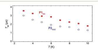
Fig. 7 Temperature dependence of the quantum coherence time  $T_{\rm M}$  for P1<sub>Gd</sub> (red full dots) and P2<sub>Gd2</sub> (blue empty dots), as measured at 344 mT at 9.37 GHz in a 1:1 mixture of dichloromethane and toluene.
