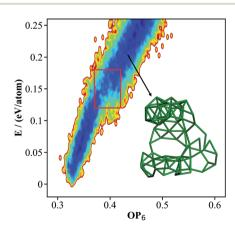
Fig. 3 The contour map (E against OP<sub>6</sub>, also see Fig. 1 caption for explanation) for the  $\beta$ -B minima from the SSW global optimization using the boron NN PES. The red box indicates the boundary above which the  $B_{28}$  cages start to melt. The inset shows a typical structure with broken  $B_{28}$  cages.
