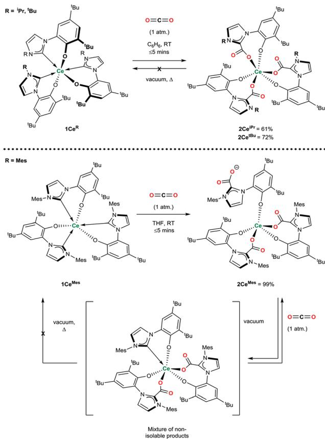
Scheme 2 Reactivity of  $1\text{Ce}^{\text{R}}$  with  $\text{CO}_2$  that forms the triply  $\text{CO}_2$ -NHC inserted adducts irreversibly ( $2\text{Ce}^{\text{iPr}}$  and  $2\text{Ce}^{\text{tBu}}$ ) and reversibly ( $2\text{Ce}^{\text{Mes}}$ ).
