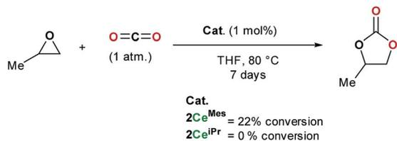
Scheme 5 Catalytic formation of propylene carbonate from propylene oxide in an atmosphere of carbon dioxide using 2Ce<sup>Mes</sup> and 2Ce<sup>iPr</sup>.
