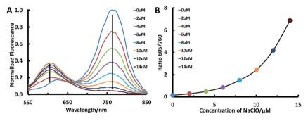
Fig. 1 (A) Emission spectra of CIO1 (5  $\mu$ M) upon treatment with various concentrations of NaClO (0-14  $\mu$ M); (B) fluorescence ratio ( $I_{605}/I_{760}$ ) of ClO1 (5  $\mu$ M) upon treatment with various concentrations of NaClO (0–14  $\mu$ M).
