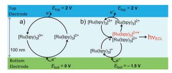
Fig. 2 Schematic of two reaction pathways in the nanochannel: (a) redox cycling, and (b) annihilation leading to ECL emission.
