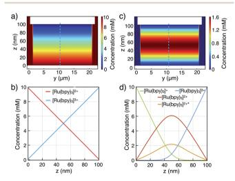
Fig. 5 Finite element simulations of concentration profiles for a 10 mM  $[Ru(bpy)_3]^{2+}$  bulk concentration in the nanochannel. Two-dimensional  $[Ru(bpy)_3]^{2+}$  profiles in (a) redox cycling mode, and (c) annihilation mode. (b and d) Corresponding cross-sectional profiles in the channel center (indicated by the dashed line in both modes, respectively).
