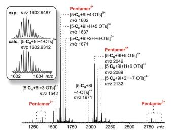
Fig. 5 ESI-Q-TOF-HRMS spectrum of pentameric halogen-bonded capsule 3 (90  $\mu$ M in CH<sub>2</sub>Cl<sub>2</sub>) with experimental and calculated isotopic pattern (inset).
