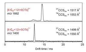
Fig. 3 DT-IM-MS ATDs of ions derived from hexameric halogenbonded capsule 2. Experimental DTCCS<sub>He</sub> and theoretical TMCCS<sub>He</sub> values are given.
