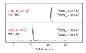
Fig. 1 DT-IM-MS ATDs of ions derived from dimeric halogen-bonded capsule **1**. Experimental <sup>DT</sup>CCS<sub>He</sub> and theoretical <sup>™</sup>CCS<sub>He</sub> values are given.
