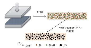
Fig. 1 Illustration of the preparation process of carbon supported Li–Si alloy electrodes.
