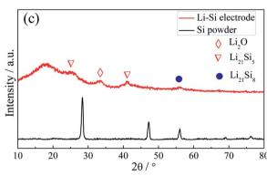
Fig. 2 The photo images of a fresh pressed Li–Si–CNF composite (a) and a heat treated Li–Si alloy electrode (b), and the XRD patterns of Si powder and the Li–Si alloy electrode (c).
