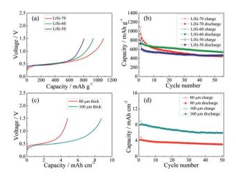
Fig. 4 The initial charge curves (a) and cycling performance (b) of the Li–Si alloy electrode with 50, 60 and 70 wt% Li–Si (0.01–1.5 V, 100 mA  $\rm g^{-1}$ ); the initial charge curves (c) and cycling performance (d) of the Li–Si alloy electrode containing 60 wt% Li–Si with different thicknesses (0.01–1.5 V, 100 mA  $\rm g^{-1}$ ).
