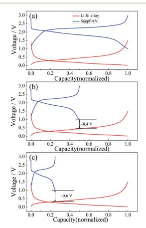
Fig. 6 The normalized charge/discharge curves of the Li-S@pPAN cell (1C) and Li-Si alloy electrode (100 mA  $g^{-1}$ ) with anode to cathode capacity ratios of 1:1 (a), 2:1 (b) and 4:1 (c).
