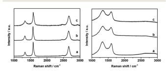
Fig. 1 Representative Raman spectra collected at different regions of the samples GR-BZ (a), GR-BZ/HX (b) and GR-HX (c).
