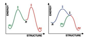
Fig. 1 Schematic representations of a reaction with two products, each formed *via* a different TSS (left) and a reaction with a PTSB (right). For the latter, it is inappropriate, but convenient for purposes of illustration, for both the green and red portions of the reaction coordinate to be projected into the same two dimensions as the blue portion.
