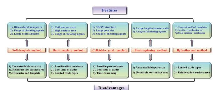
Fig. 4 Summary of synthesis methods for nanoporous perovskite metal oxides.
