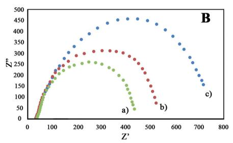
Fig. 7 (A) TGA patterns of (a) Ti, (b) ZnTi, and (c) GZnTi; (B) EIS spectra of (a) Ti, (b) ZnTi, and (c) GZnTi catalysts under visible light irradiation.
