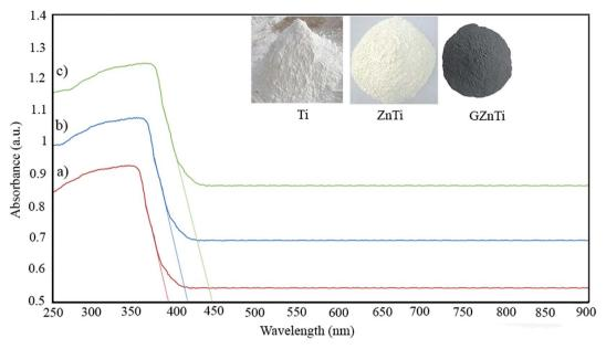
Fig. 4 UV-visible adsorption spectra of (a) Ti, (b) ZnTi, and (c) GZnTi.
