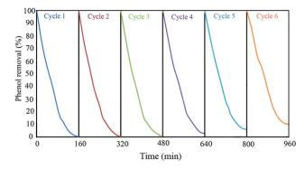
Fig. 9 Recyclability of GZnTi in Ph-degradation process in the presence of visible light illumination through 6 cycles at pH: 4, catalyst dosage:  $0.6 \, \mathrm{g \, L^{-1}}$ , and phenol concentration: 60 ppm (at the optimum Ph-degradation conditions).
