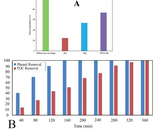
Fig. 10 (A) Ph-degradation efficiency in the presence of different radical scavengers (IPA, BZQ, Na<sub>2</sub>-EDTA); (B) comparison of phenol removal and TOC removal at pH: 4, catalyst dosage:  $0.6 \text{ g L}^{-1}$ , and phenol concentration: 60 ppm.
