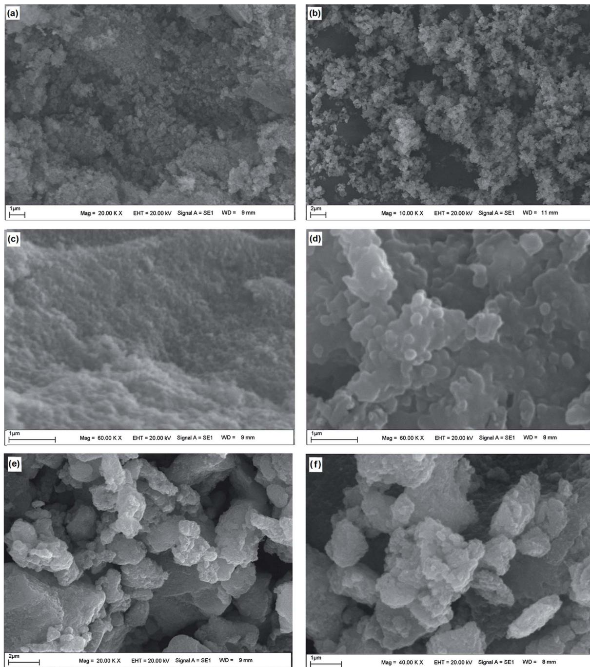
Fig. 9 SEM analysis of magnetic (a and c)  $\text{Fe}_3\text{O}_4$ , (b and d)  $\text{Fe}_3\text{O}_4$ -chitosan particles and (e and f)  $\text{Fe}_3\text{O}_4$ -chitosan-L-ASNase at different magnifications.
