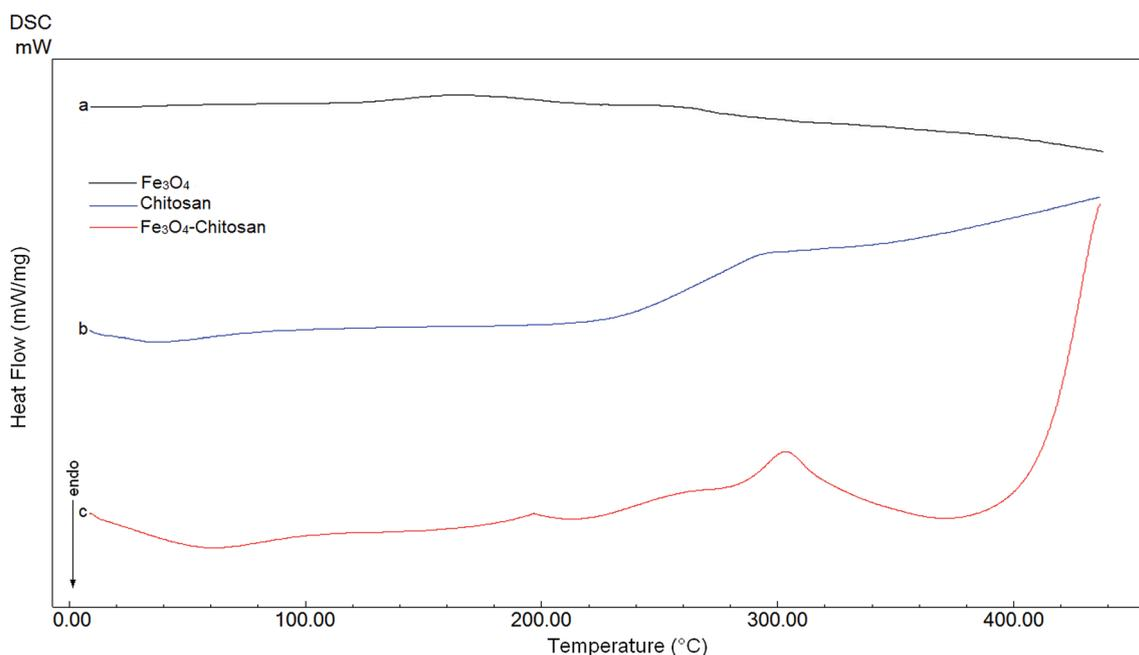
Fig. 6 DSC curves of (a) Fe<sub>3</sub>O<sub>4</sub>, (b) chitosan, and (c) Fe<sub>3</sub>O<sub>4</sub>-chitosan particles.
