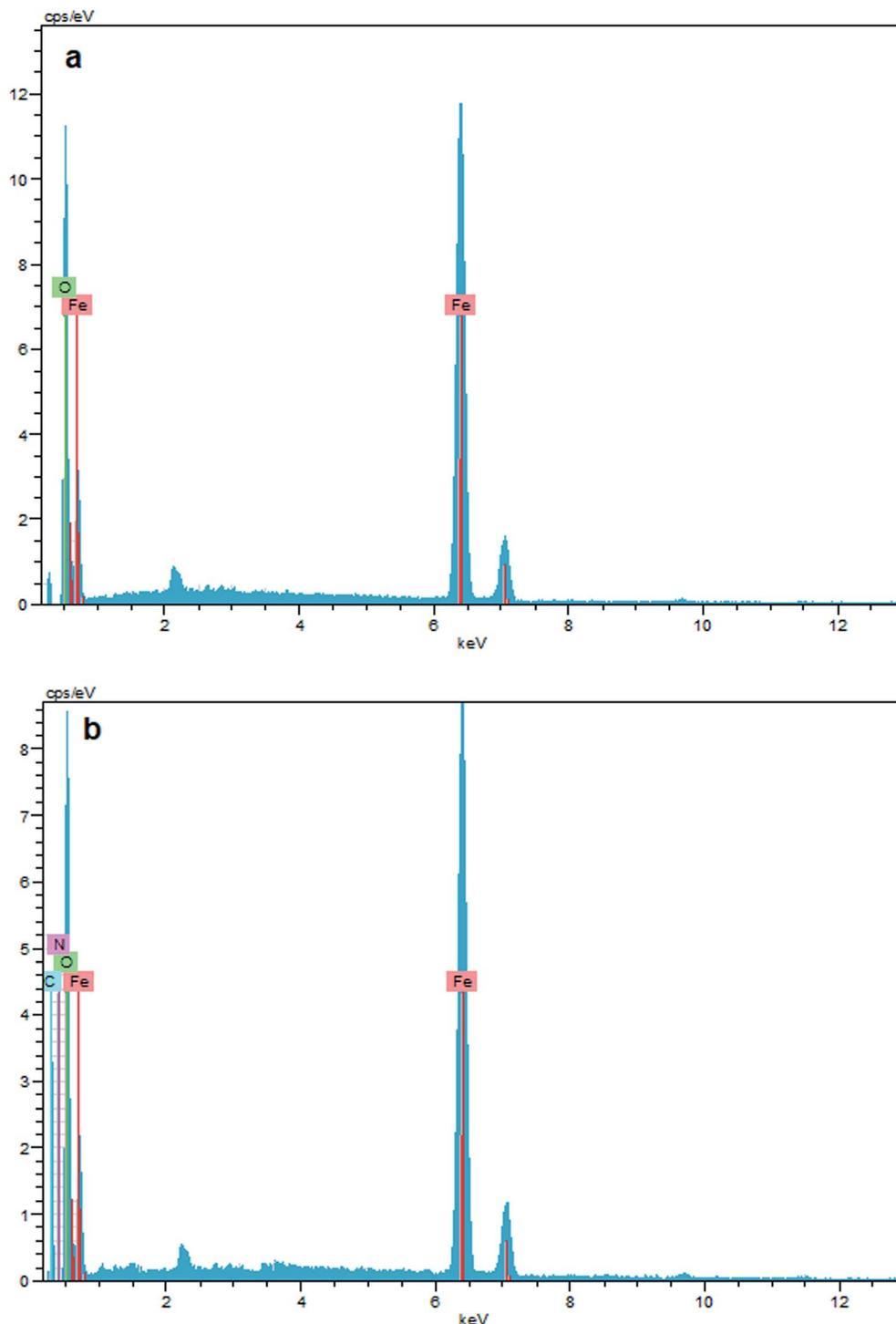
Fig. 10 EDX result of (a) Fe<sub>3</sub>O<sub>4</sub>, and (b) Fe<sub>3</sub>O<sub>4</sub>-chitosan particles.
