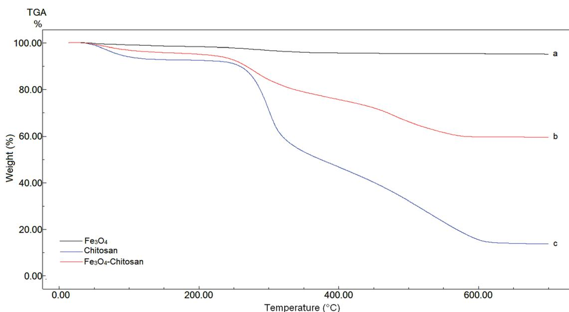
Fig. 4 TGA curves of (a) Fe<sub>3</sub>O<sub>4</sub>, (b) chitosan, and (c) Fe<sub>3</sub>O<sub>4</sub>-chitosan particles.
