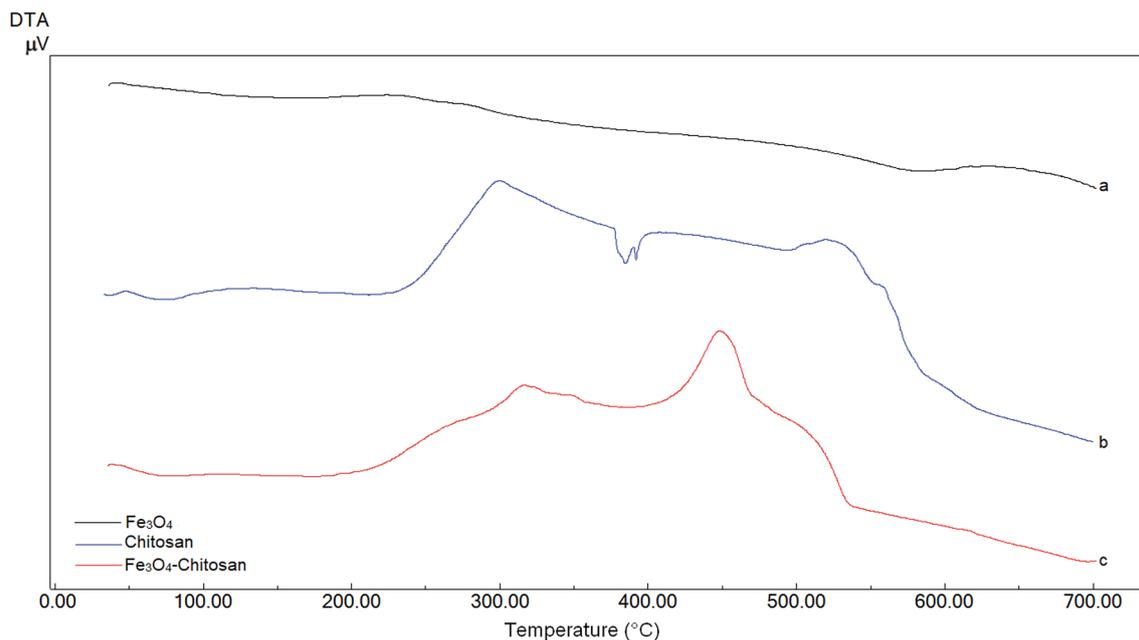
Fig. 5 DTA curves of (a) Fe<sub>3</sub>O<sub>4</sub>, (b) chitosan, and (c) Fe<sub>3</sub>O<sub>4</sub>-chitosan particles.
