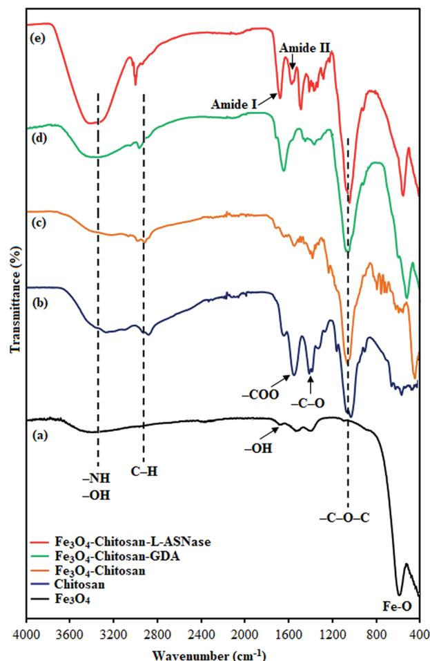
Fig. 3 FTIR spectra of (a) Fe<sub>3</sub>O<sub>4</sub>, (b) chitosan, (c) Fe<sub>3</sub>O<sub>4</sub>-chitosan particles, (d) Fe<sub>3</sub>O<sub>4</sub>-chitosan-GDA, and (e) Fe<sub>3</sub>O<sub>4</sub>-chitosan-L-ASNase.
