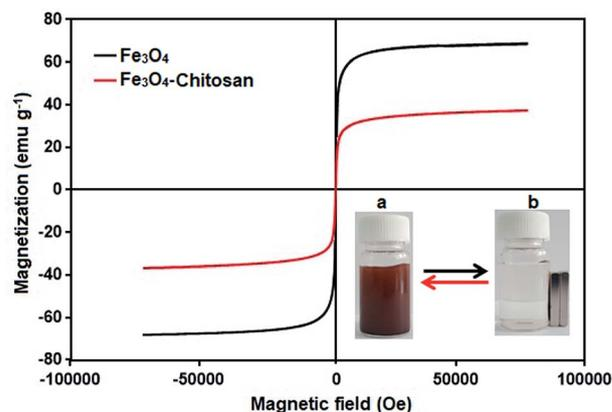
Fig. 11 VSM measurements of the obtained  $\text{Fe}_3\text{O}_4$  and  $\text{Fe}_3\text{O}_4$ -chitosan particles. The photographic image of  $\text{Fe}_3\text{O}_4$ -chitosan particles (a) without magnet and (b) with magnet.
