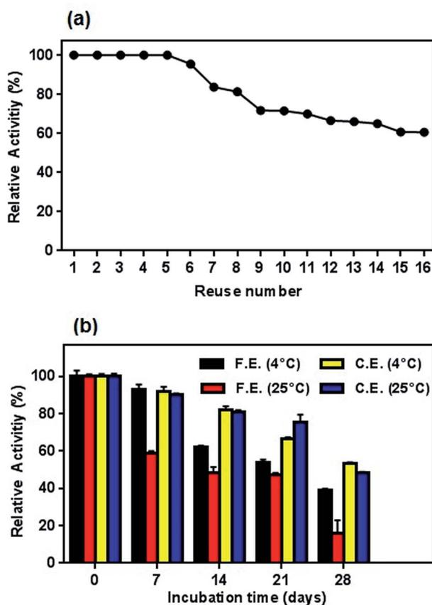
Fig. 14 (a) Profile of reusability test for conjugated enzyme and (b) storage stability of free and conjugated L-ASNase on Fe<sub>3</sub>O<sub>4</sub>-chitosan at 4 °C and r.t. in dried state.
