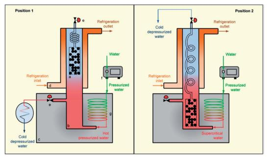
Fig. 6 Scheme of a supercritical regeneration setup, including sample holder (a), reactor (b) and (c), oven refrigeration jacket (d), system of pressure regulating valves (e), dosing pump (g), preheater (f). This figure has been adapted/reproduced from ref. 163 with permission from Elsevier.
