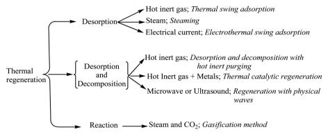
Fig. 7 Classification of thermal regeneration methods.
