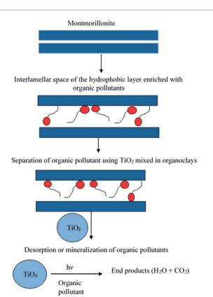
Fig. 8 Scheme for the photocatalytic regeneration of dye pollutants using  $TiO_2$ . This figure has been adapted/reproduced from ref. 179 with permission from Taylor & Francis.
