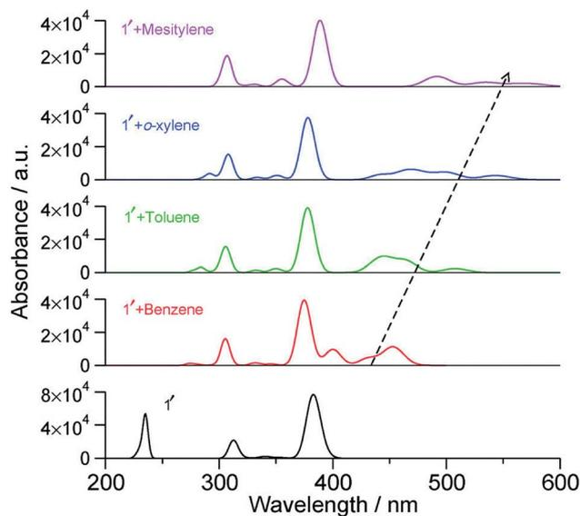
Fig. 10 Calculated vertical transitions of NDI derivative-solvent complexes at the BLYP-D3/DZVP//B3LYP/6-31+G(d,p) level of theory (fwhm = 1000  $\text{cm}^{-1}$ ). The black dashed arrow indicates the changes in the CT transition with increasing electron donating capacity of the solvent molecule. This figure has been reproduced from ref. 69 with permission from the PCCP Owner Societies.
