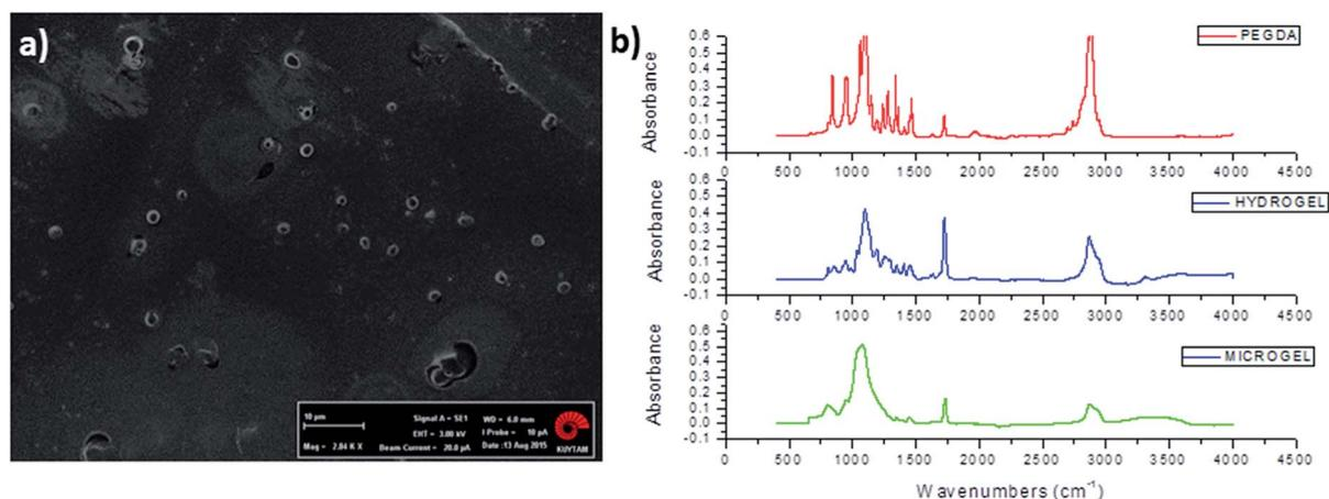
Fig. 3 Structural characterization of PEG particles. (a) SEM image of casted PEG particles (scale bar: 10  $\mu\text{m}$ ) (b) FTIR spectra of PEGDA, PEG bulk hydrogel and PEG microgel.
