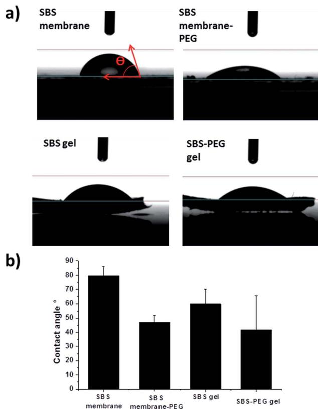
Fig. 6 Water contact (a) images and (b) angles ( $\theta$ ) of SBS membrane, SBS gel, SBS membrane-PEG and SBS-PEG gel surfaces. 10  $\mu$ L of deionized, triple distilled water was placed on surfaces for the measurement of contact angles.
