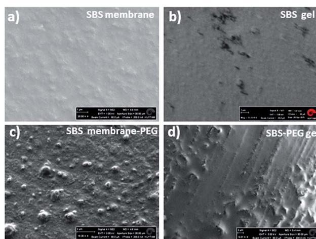
Fig. 5 SEM images of (a) SBS membrane (scale bar 1  $\mu\text{m}$ ) (b) SBS gel (scale bar 1  $\mu\text{m}$ ) (c) SBS membrane-PEG (scale bar 2  $\mu\text{m}$ ) and (d) SBS-PEG gel (scale bar 2  $\mu\text{m}$ ). SBS membrane-PEG gels were prepared by casting SBS solution after incorporation of PEG particles. SBS gel and SBS-PEG gel were prepared by crosslinking of SBS solution after incorporation of PEG particles. Hybrid gels were dried in vacuum oven overnight before analysis with SEM.
