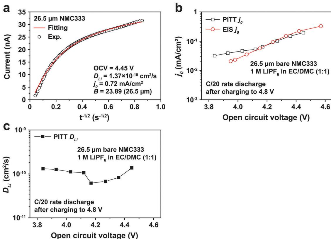
Fig. 5 (a) PITT current vs. time data, and corresponding least-squares fit to eqn (5), from which kinetic parameters are obtained, for an NMC333 particle of 26.5  $\mu\text{m}$  diameter, measured for a +15 mV voltage step from a relaxed OCV of 4.45 V. (b) The dependence of  $j_0$  on OCV from PITT (black squares) is in good agreement with those obtained from EIS (red circles). (c) Chemical diffusion coefficient  $D_{Li}$  vs. OCV, based on PITT measurements.
