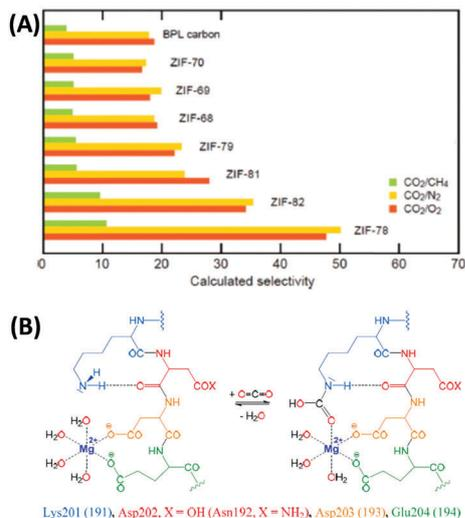
Fig. 3 (A) CO<sub>2</sub>/CH<sub>4</sub>, CO<sub>2</sub>/N<sub>2</sub>, and CO<sub>2</sub>/O<sub>2</sub> selectivities of different zeolitic imidazole frameworks (ZIFs) showing that the CO<sub>2</sub>/N<sub>2</sub> and CO<sub>2</sub>/O<sub>2</sub> selectivities follow the same trends.<sup>30</sup> (B) CO<sub>2</sub> capture in the active site of rubisco.<sup>40</sup> (A) Reproduced with permission from ref. 30. Copyright (2009) American Chemical Society.
