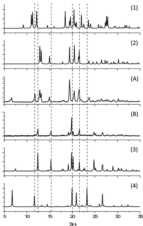
Fig. 6 (A) XRPD pattern of  $\epsilon$ -CPA after impact treatment with heptane, (B) XRPD pattern of  $\beta$ -CPA converted into  $\gamma$ -form after shear treatment with heptane, and simulated XRPD patterns for (1)  $\beta$ -CPA, (2)  $\epsilon$ -CPA, (3)  $\gamma$ -CPA and (4)  $\delta$ -CPA.
