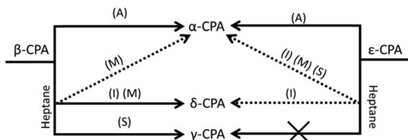
Fig. 5 Schematic summary of the mechanically-induced transformations of  $\varepsilon$ - and  $\beta$ -CPA. (A) Transformation observed under all types of mechanical treatment in the presence of moisture, ethanol, chloroform or toluene. Specific reactivity under restricted impact (I), manual grinding (M) or shear (S) are indicated for LAG with heptane.
