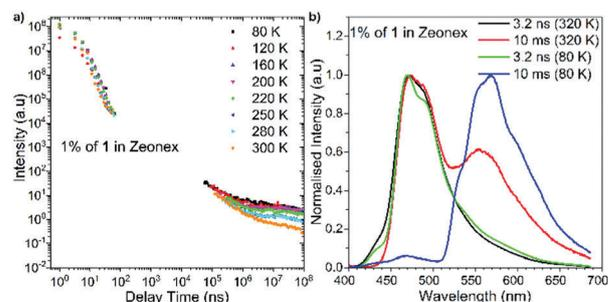
Fig. 5 (a) Temperature-variable plots of emission intensity of **1** in Zeonex<sup>®</sup> (1% w/w) against delay time at different temperatures; (b) normalized PL spectra of **1** in Zeonex<sup>®</sup> at 320 K and 80 K.
