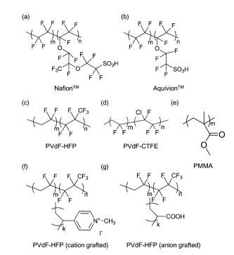
Fig. 2 Chemical structures of various polymers that have been employed for IPMC actuators: (a) Nafion™, (b) Aguivion™, (c) PVdF-HFP, (d) PVdF-CTFE, (e) PMMA, (f) cation-grafted PVdF-HFP, and (g) anion-grafted PVdF-HFP. (f) and (g) are reproduced from ref. 40 with the permission of American Chemical Society.
