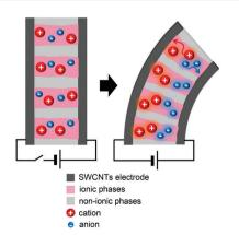
Fig. 6 Schematic illustration of the electromechanical actuation mechanism for the actuators comprising self-assembled block copolymer electrolytes under an applied voltage.
