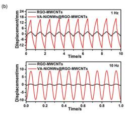
Fig. 5 (a) Schematic illustration of the structure and assembly procedure of the actuators based on a hierarchically architectured electrode. (b) Comparison of the bending performance of the actuators with and without vertically aligned NiO nanowires with an applied voltage of 2.5 V with frequencies of 1 Hz and 10 Hz. Figure is reproduced from ref. 65 with the permission of Royal Society of Chemistry.
