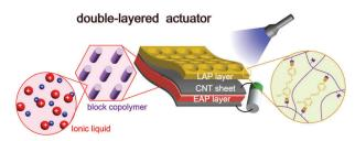
Fig. 9 Schematic illustration of light- and electro-active polymer actuators based on the double-layered structures. Figure is reproduced from ref. 89 with the permission of Wiley-VCH.
