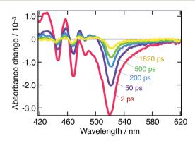
Fig. 2 Transient absorption spectra of a suspension of  $CH_3NH_3PbBr_3$  nanoparticles in chlorobenzene at different time delays following  $\lambda_{\rm ex}=390$  nm pulsed excitation. Red: t=2 ps, purple: t=50 ps, blue: t=200 ps, green: t=500 ps, and yellow: t=1820 ps.
