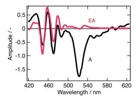
Fig. 5 Modeled electroabsorption signal of a suspension of  ${\rm CH_{3^-}NH_{3}PbBr_{3}}$  nanoparticles in chlorobenzene. The blue part of the observed transient absorption spectrum measured at a time delay of 2 ps (black line) fits well with a simulated electroabsorption spectrum (red) dominated by the second derivative component of the ground state absorption spectrum (see ESI† for details).
