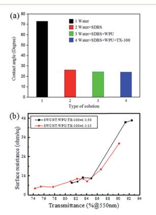
Fig. 2 (a) Effect of different additives on the contact angle of the suspension; (b) the film surface resistance as a function of transmittance with different contents of TX-100, and the points were obtained by changing the dilution of the CNT suspension and the wire diameters
