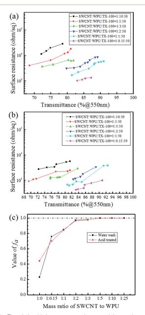
Fig. 3 The relationship between transmittance and sheet resistance of (a) water washed CNT-TAFs and (b) acid treated CNT-TAFs, the points were obtained by changing the dilution of the CNT suspension and wire diameters; (c) adhesion factor  $(f_a)$  at different mass ratios of SWCNT to WPU.
