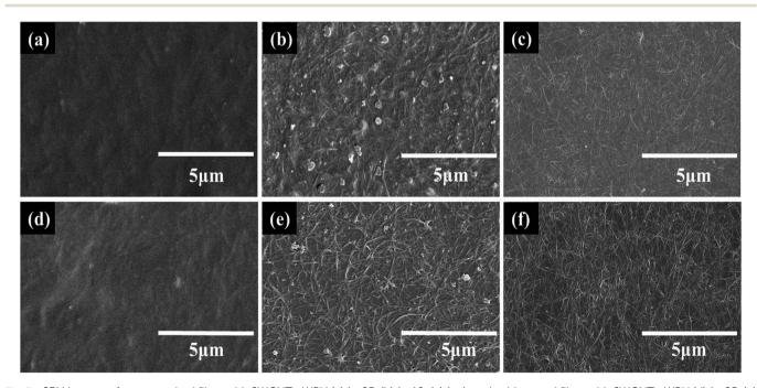
Fig. 5 SEM images of water washed films with SWCNT: WPU (a) 1:25, (b) 1:10, (c) 1:1, and acid treated films with SWCNT: WPU (d) 1:25, (e) 1:10, (f) 1:1.
