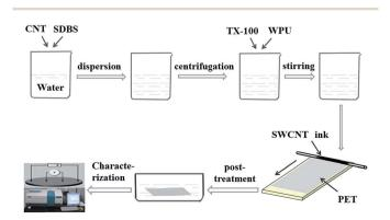
Fig. 1 Schematic about preparation of CNT suspension, coating method, post-treatment and characterization of TAFs.
