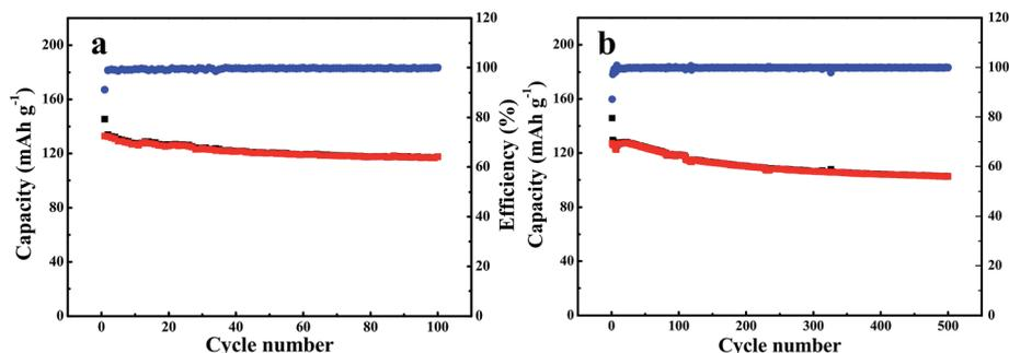
Fig. 10 Cycling performance of LiFePO<sub>4</sub>/GPE/Li battery testing at current density of (a) 0.5C, (b) 0.2C.
