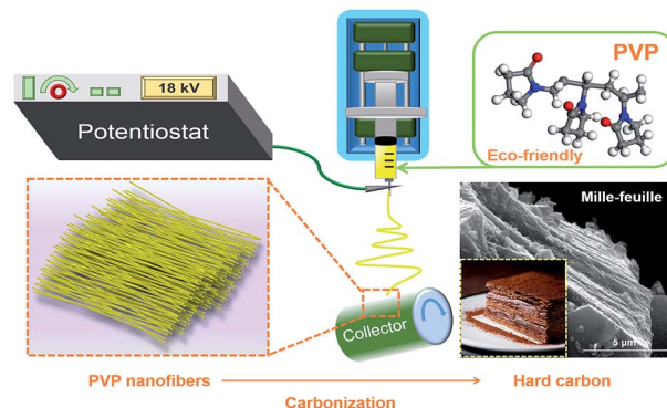
Scheme 2 Schematic illustration of the synthesis process for the mille-feuille shaped hard carbons derived from PVP.
