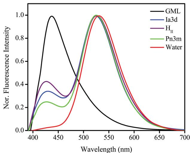
**Fig. 2** Normalized (normalized with respect to  $Z^*$  emission maximum) steady state emission spectra of TPT in bulk water, GML and inside *Pn3m*, *Ia3d* and  $H_{\text{II}}$  LLC phases ( $\lambda_{\text{ex}} = 380$  nm).
