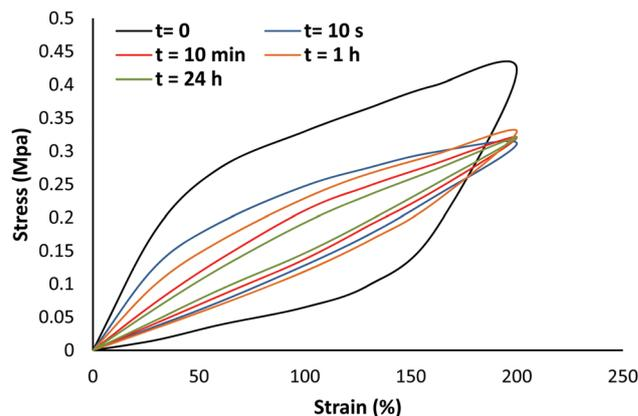
Fig. 9 Hysteresis effect of loading to a certain stretch ( $\lambda = 4$ ) and unloading to zero for first and second loadings with different time intervals. All dynamic tests were performed at  $50 \text{ mm min}^{-1}$  strain rate.
