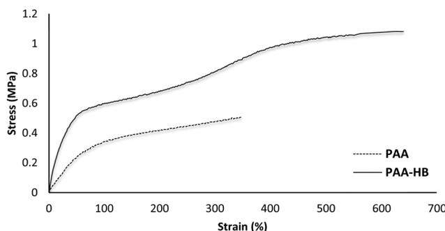
Fig. 6 Mechanical properties of PAA and PAA-HB hydrogels.
