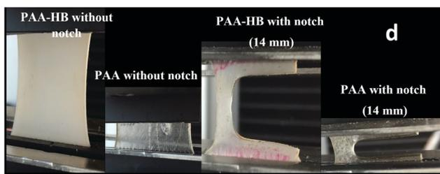
Fig. 8 Comparison of the mechanical properties of PAA with PAA-HB hydrogel for different notch depths. (a) Ultimate tensile strength, (b) elongation at break and (c) toughness. Figure (d) shows the stretchability of the intact sample (un-notched) versus the notched sample (14 mm) for both PAA and PAA-HB hydrogels.
