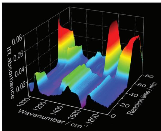
Fig. 4 Time-dependence of *in situ* IR spectroscopy measurements during the synthesis of Ce<sup>3+</sup>-doped calcium phosphate (experiment 2, Table 1).
