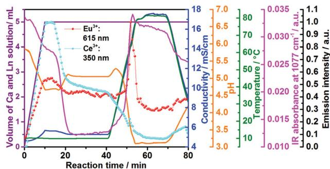
Fig. 3 Time dependence of the emission intensity of  $\text{Ce}^{3+}$  (light blue curve) and  $\text{Eu}^{3+}$  (red curve) doped calcium phosphate, *in situ* ion conductivity (dark blue curve), *in situ* pH (orange curve) and IR intensity at  $1077\text{ cm}^{-1}$  (pink curve) in comparison with the volume of the  $\text{Ca}^{2+}$  and  $\text{Ln}^{3+}$  solution (violet curve) to the reactor containing aqueous  $(\text{NH}_4)_2\text{HPO}_4$  (experiments 2 and 6, Table 1).
