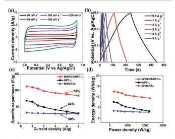
Fig. 10 Electrochemical performances evaluated by symmetrical twoelectrode supercapacitors in 1 M H<sub>2</sub>SO<sub>4</sub> solution. (a) CV curves of MWCNT/NPC-L-based SSC at different scan rates. (b) Charge-discharge curves of MWCNT/NPC-L-based SSC at various current densities. (c) Specific capacitance under different current densities from 0.5 to 5 A g<sup>-1</sup>. (d) Ragone plot for the SSCs based on MWCNT/NPC-L, NPC-L and MWCNTs under various current densities.
