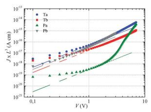
Fig. 2 Space-charge-limited current on as-cast polymers. For  $\mathbf{P_a}$  the curve has been obtained by averaging the current-voltage data of four devices processed under identical conditions. The dashed lines correspond to a fit in the voltage range where J follows a square-law dependence (constant mobility) on the voltage.
