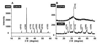
Fig. 3 XRD pattern obtained from (A) calcite and (B) the two  $CaCO_3$  preparations, containing two different concentrations of polyP, "CCP5" or "CCP10". The characteristic signals are highlighted and marked with the respective Miller indices, given in parentheses.<sup>36</sup> Please note the different scale of the ordinate captions between (A) and (B).
