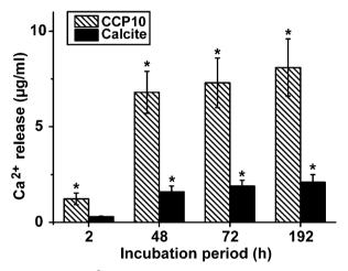
Fig. 7 Release of Ca<sup>2+</sup> from the CaCO<sub>3</sub> particles. "CCP10" or calcite was incubated in Tris-HCl buffer (pH 7.4) for various time periods and the supernatant was analyzed for Ca<sup>2+</sup> concentration. The results are means from 6 parallel experiments; \*P < 0.01.
