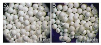
Fig. 9 Morphology of the microspheres; (A) control spheres "cont-mic" and (B) polyP loaded spheres, "polyP-mic".
