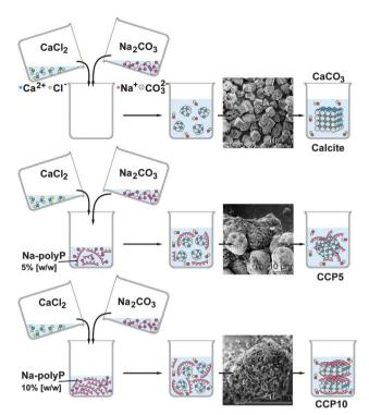
Fig. 1 Preparation of calcite and CaCO<sub>3</sub> supplemented with polyP (scheme). The insets show the SEM images of the respective product.
