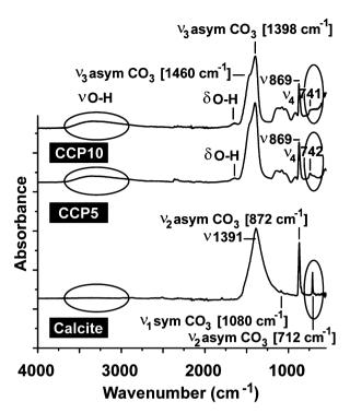
Fig. 2 FTIR spectra of calcite as well as "CCP5" (0.05 g of Na-polyP/assay) and "CCP10" (0.1 g of Na-polyP). The major distinguishing vibration regions/ signals for calcite *versus* ACC, the vibration range for O-H (around  $3250 \text{ cm}^{-1}$ ) and the asymmetric  $v_2$  line for CO<sub>3</sub> at  $712/742 \text{ cm}^{-1}$  are circled.
