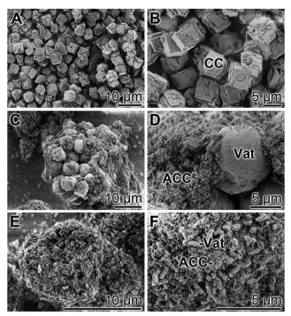
Fig. 4 Morphology of the solids formed from  $CaCl_2 \cdot 2H_2O$  and  $Na_2CO_3$ ; SEM analysis. (A and B) In the absence of polyP calcite crystals are formed. This morphology is changed after the addition of polyP during the precipitation process. (C and D) In the presence of 5% polyP, the "CCP5" particles show a spherical appearance. (E and F) At 10% polyP, "CCP10", the solids show a platelet-like shape, which corresponds to vaterite crystals (Vat).
