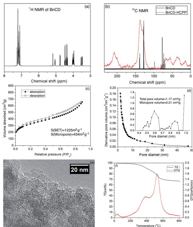
Fig. 1 (a)  $^1\text{H}$  NMR spectrum of BnCD, (b)  $^{13}\text{C}$  NMR of BnCD and solid-state  $^{13}\text{C}$  NMR of BnCD-HCPP (spinning at 7 K), (c)  $\text{N}_2$  adsorption–desorption isotherms of BnCD-HCPP measured at 77 K (the polymer was pretreated at 170 °C under nitrogen flow for 2 h), (d) pore size distribution of BnCD-HCPP, (e) transmission electron microscope image of BnCD-HCPP, and (f) thermogravimetry and differential thermogravimetry curves of BnCD-HCPP.
