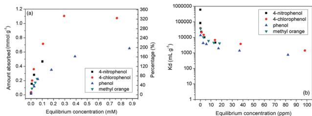
Fig. 2 Adsorption isotherms (a) and distribution coefficient (b) of BnCD-HCPP toward *p*-nitrophenol, *p*-chlorophenol, phenol, and methyl orange. The percentage in (a) was calculated as a molar percentage (mol/mol%) of the absorption amount (mmol g<sup>-1</sup>) to the amount of CD units (mmol g<sup>-1</sup>) in the adsorbent.
