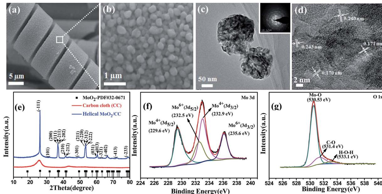
Fig. 3 (a and b) SEM images of the helical  $\text{MoO}_2$  with different magnifications; (c) the TEM image of  $\text{MoO}_2$  nanoparticles (inset is the SAED pattern); (d) the HRTEM image of the helical  $\text{MoO}_2$ ; (e) XRD patterns of the helical  $\text{MoO}_2/\text{CC}$  and CC; XPS spectra of the helical  $\text{MoO}_2/\text{CC}$ : (f) Mo 3d and (g) O 1s.
