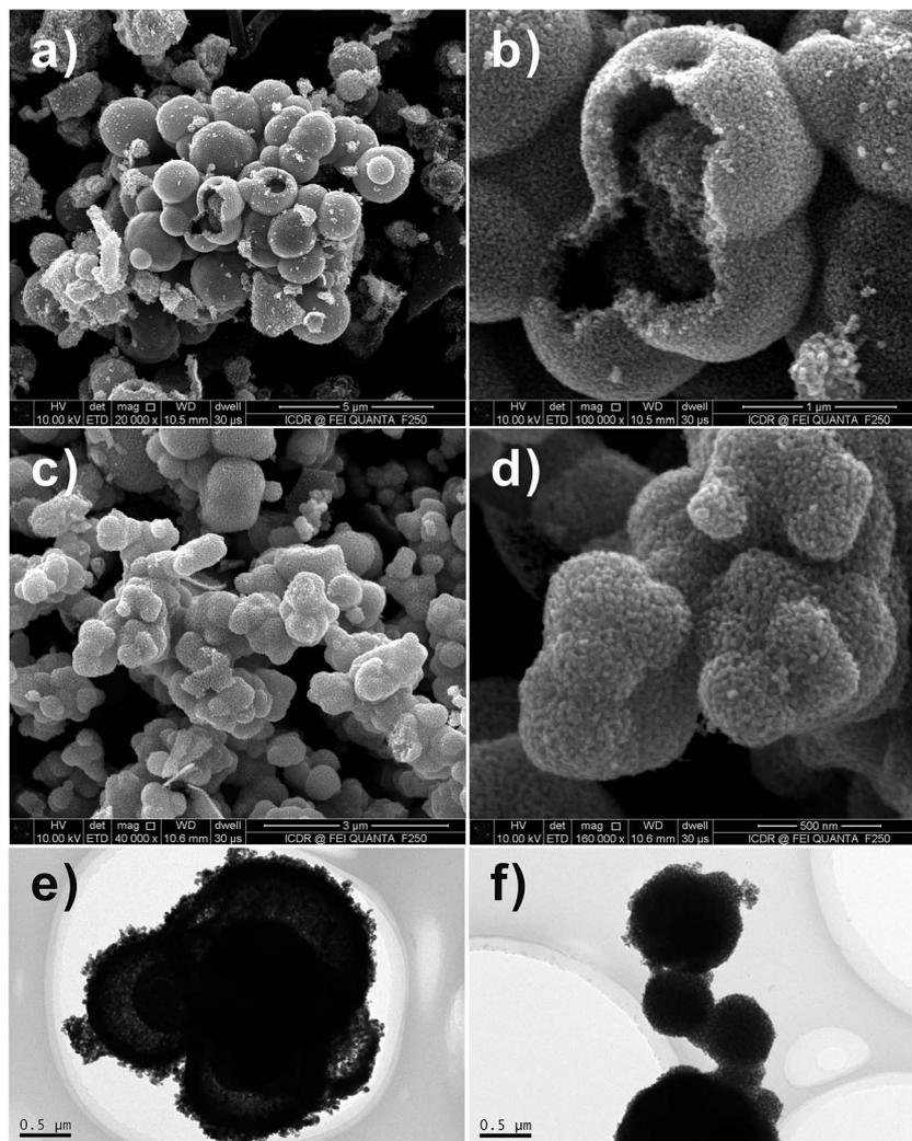
Fig. 6 FESEM and TEM images of  $\text{SnO}_2$  samples after calcination at  $600^\circ\text{C}$  for 3 h with (a and b, e) 2 : 1 and (c and d, f) 1 : 2 molar ratio of D-glucose and  $\text{SnCl}_4 \cdot 5\text{H}_2\text{O}$ .
