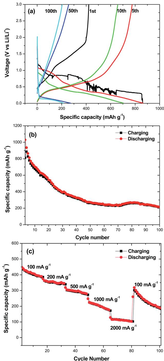
Fig. 8 (a) Charge–discharge curves of the multi-shelled  $\text{SnO}_2$  hollow sphere electrode for the 1<sup>st</sup>, 5<sup>th</sup>, 10<sup>th</sup>, 50<sup>th</sup>, and 100<sup>th</sup> cycle at current density of  $100 \text{ mA g}^{-1}$ ; (b) the cycling performance of the multi-shelled  $\text{SnO}_2$  hollow spheres; (c) charge–discharge curves of the multi-shelled  $\text{SnO}_2$  hollow spheres at different current densities.
