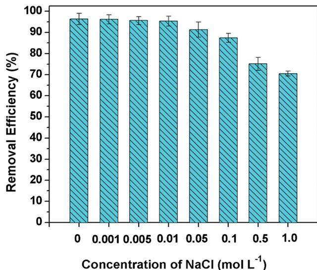
Fig. 9 Effect of different concentrations of NaCl on Cr(vi) removal by  $\beta$ -CCWB450 (Cr(vi) solution volume: 50 mL; adsorbent dose: 0.1 g; initial Cr(vi) concentration: 100 mg L<sup>-1</sup>; contact time: 24 h; pH: 2.0).
