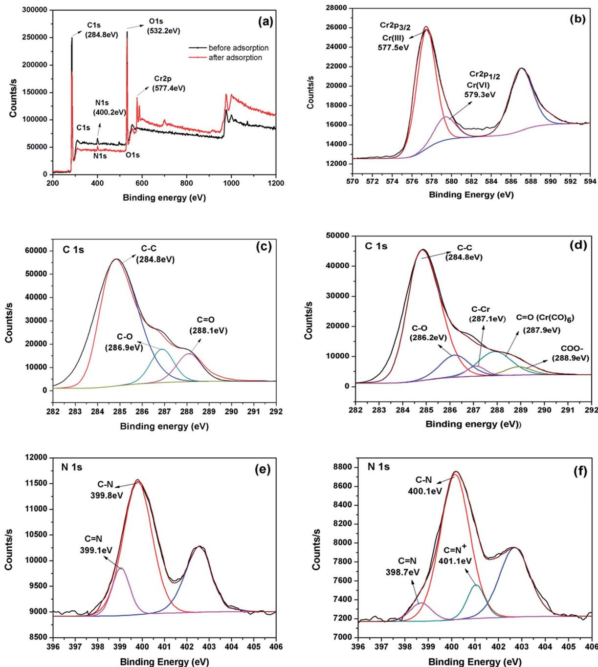
Fig. 3 XPS spectra of (a)  $\beta$ -CCWB450 before and after adsorption, (b) Cr<sub>2p</sub> of  $\beta$ -CCWB450 after adsorption, (c) the C 1s XPS spectra of  $\beta$ -CCWB450 before and (d) after adsorption, (e) the N 1s XPS spectra of  $\beta$ -CCWB450 before and (f) after adsorption.
