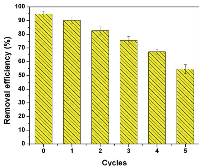
Fig. 10 Fifth consecutive adsorption–desorption cycles of  $\beta$ -CCWB450 for Cr(vi) removal (Cr(vi) solution volume: 50 mL; adsorbent dose: 0.1 g; initial Cr(vi) concentration: 100 mg L<sup>-1</sup>; contact time: 24 h; pH: 2.0).
