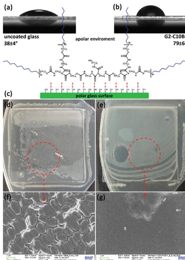
**Fig. 8** Contact angle of a water droplet on a glass slide before (a) and after (b) coating with G2-C10Br. A crude model for the conformation of G2-C10Br dendrons on a polar surface (c). Pictures and SEM images for uncoated (d, f) and coated (e, g) glass slides contacted with *E. coli* ( $10^6$  CFU) after incubation at 37 °C overnight. SEM images are at 10 000 magnifications.
