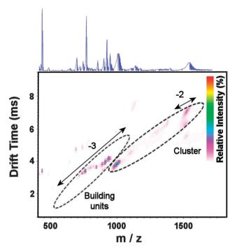
Fig. 3 ESI-IMS-MS of  $\{Mo_{16}\}$  1 in MeOH. Relative intensity (*cf.* highest peak) is shown on a linear scale (coloured scale, inset); samples of isotope patterns (inset) were obtained in resolution mode; see ESI† for details.
