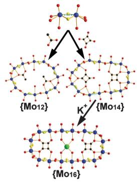
Fig. 2 Templated directed assembly of [Mo<sub>2</sub>O<sub>2</sub>S<sub>2</sub>]<sup>2+</sup> dimeric units leading to 1 (Mo<sub>12</sub>) and (Mo<sub>14</sub>) which is transformed further to 2 (Mo<sub>16</sub>) ring associated with a 45° degree template rotation (Mo: blue; S: yellow; O: red; K: green; C: black)
